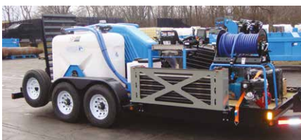
Onboard 38 l/min high pressure drill fluid pump
