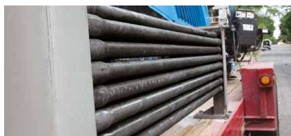
Drill rod capacity 61 metres optionally 76 metres
